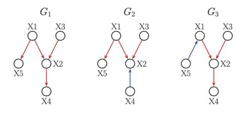
Three DAGs. G1 and G3 are Markov equivalent,G2 is not. *Graphs are Markov equivalent*
